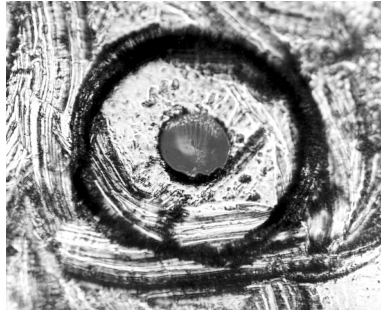
Figure 1-6. Damage from improper cleaning.
